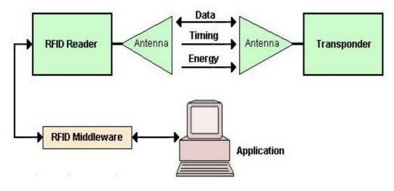
Figure 1: Components of RFID System<sup>6</sup>
